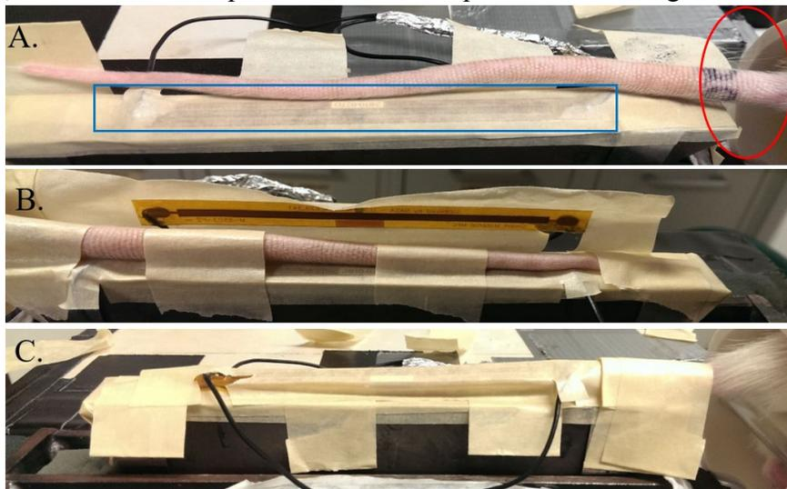
Figure 3: Step-by-step placement of the piezoelectric sensors on the vibration restraint. (A) The rat tail sits relaxed on the riveting platform. Circled in red is the fur-skin interface of the rat tail which is used to align the tail with the riveting platform. Outlined in blue is the ventral piezoelectric sensor. (B) Four tapes are placed laterally before the dorsal piezoelectric sensor is placed. (C) The dorsal piezoelectric sensor is then secured.
